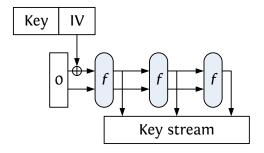
■ Encryption: add key stream to plaintext bit per bit
